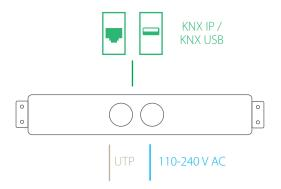
**1.Plug-in** the power supply and connect your Sledgehammer to the network via the network cable.
